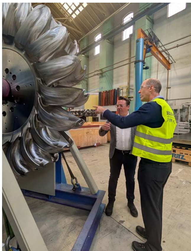
Grege Payne observing a Pelton wheel/runner used for hydro power generation at Andritz headquarters in Graz, Austria.
