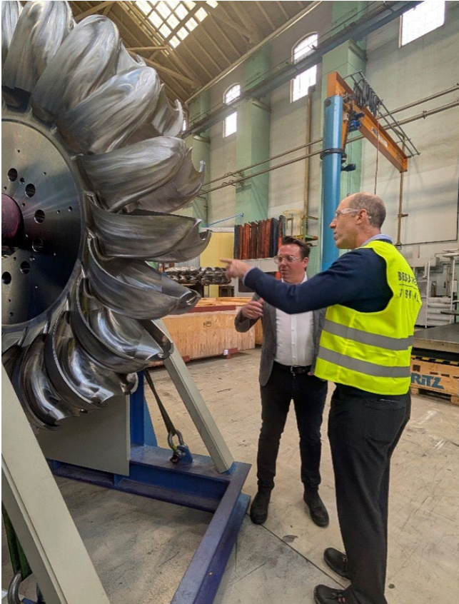
Pelton wheel/runner used for hydro power generation.
